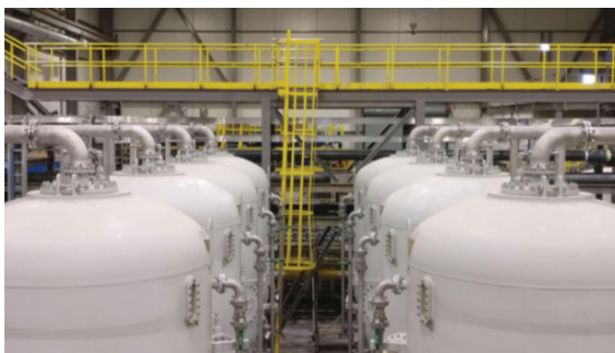
FIGURE 2. Shown here are the ion-exchange columns of the first industrial-scale Selen-IX plant
